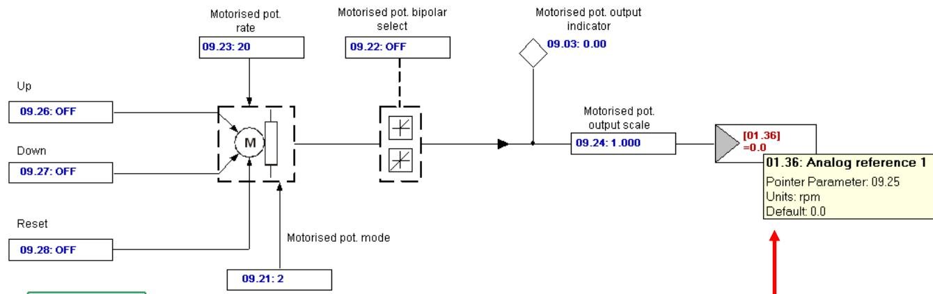
**Step 2 is to connect the output of the MOP function to the speed reference register #9.25 = 1.36**
