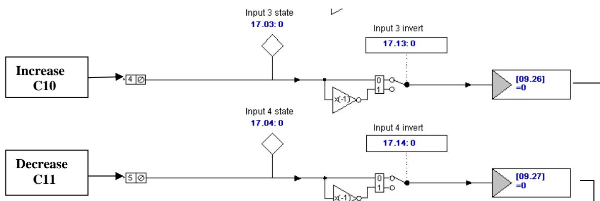
**Step 3 is to connect Terminal C10 as the Increase pushbutton by setting #17.23 to 9.26
