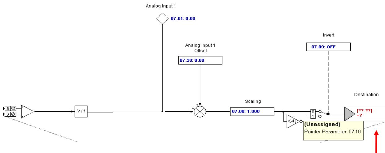
**Step 1 is to disconnect the default analog input destination by setting #7.10 = 0.00**
